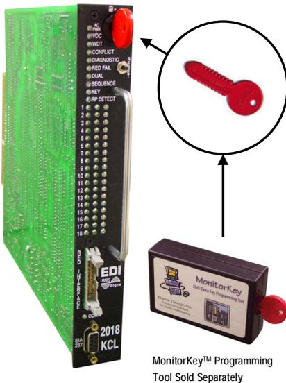
The EDI 2018KCL Signal Monitor is designed to upgrade the capabilities of the basic 210 / 2010 monitor used in Type 170 / 179 Output Files. The unit is fully compatible with the requirements of the 170, 179, and 2070 Controller Units. The 2018KCL utilizes enhanced monitoring functions to increase cabinet fault coverage, providing additional assurance that equipment malfunctions will be detected and diagnosed properly.
